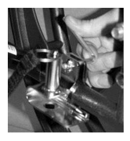
Install both brackets on the bottom horizontal tubing of the wheelchair, using an Allen Key.
