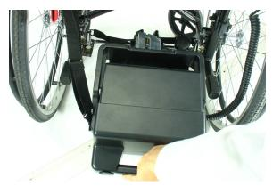
Place the battery pack in to the battery tray as shown in the photograph. Secure the battery pack on its tray.
