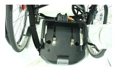
Feed the telescopic bar through the front end of the PMW-PSHD. Loosen the tristar knob on the bar and adjust to the correct length.
