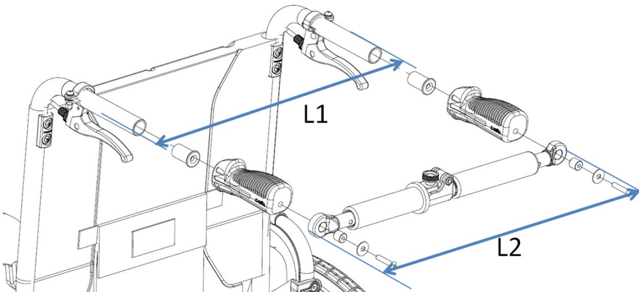
2.1. Push both lateral support bar Foam inwards until all four spring pins can be seen.
