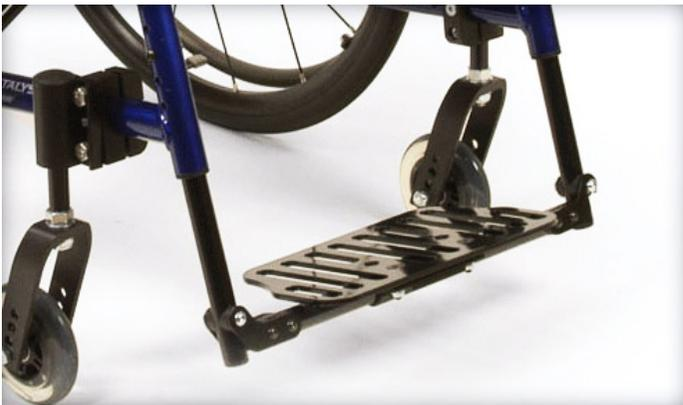
Solid, angle adjustable, aluminium footplate provides an excellent surface for your feet and increases rigidity at the front.
