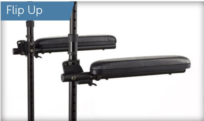
Angle Adjustable Locking Extendable Flip Up armrest is the only cantilever armrest approved to 400 lbs. Locks into position by spring loaded latch. Extends up to 4" in 1" increments and 7 angle adjustments in 5° increments from -5 to 25°. Available with standard and foam pads in desk or full lengths.
