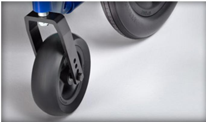
This tyre is quite firm with a subtle radius so that it is easy to push on hard surfaces and gives you great flotation on soft or uneven ground.
