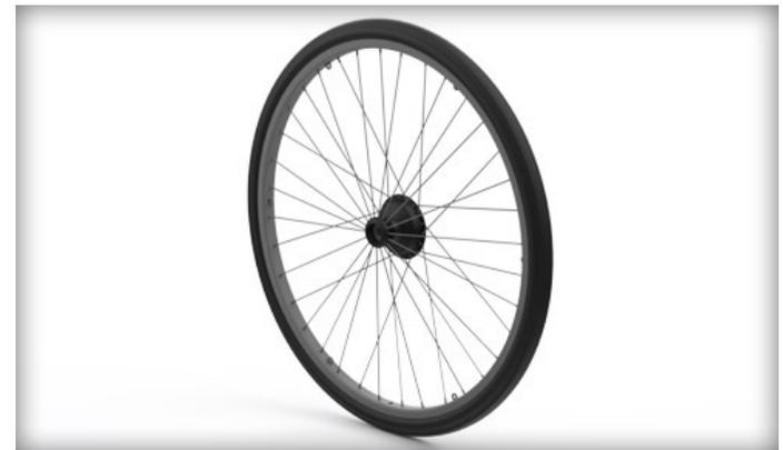
Hybrid wheel, hub design w/ straight pull radial spokes on the outside flange. Inside flange has a 2 cross spoke pattern to handle the torque resulting from stopping a larger wheel by the relatively small hub.
