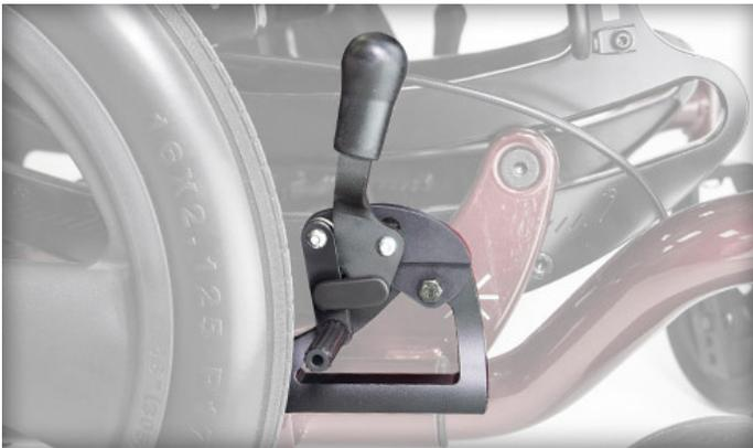
After engagement the lever is at 45 degrees. Lever is easily reachable.
