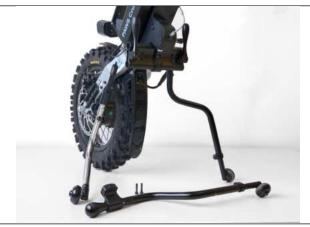
9. Here, the old support leg has been removed and the new leg has taken over the task.
