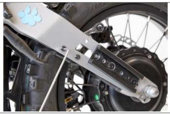
10. On the other side, you need to move the motor cable to free the screw holes to be used for the new support leg. Use a 3 mm Allen key and an 8 mm spanner to loosen both the screws for the cable.
