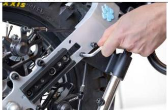
4. Tighten with a 5 mm Allen key.
