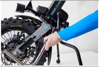
2. Insert the support leg bracket between the brake cable and the fork.
