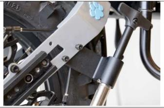
3. Use two of the screws provided to attach the support leg to the front fork.
