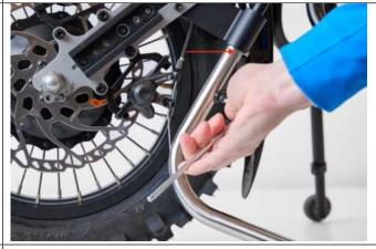
6. Loosen the screw on the support leg with a 5 mm Allen key and pull the leg down until the support wheel stands firmly on the surface. Lock the screw again.
