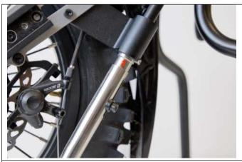
7. The picture above shows that the support leg has been extended by about one cm to allow the support wheel to make contact with the ground.
