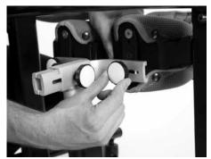
• Loosen off the turn knob under the footplate – This will then allow you to move the shoe holder in the horizontal plane in 4 directions. Set to desired position.
