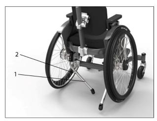
Figure 31: Deactivating/activating the anti-tipper
