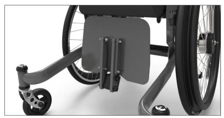
Figure 26: Foot plate, flipped up
