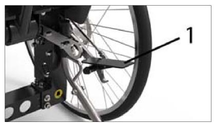
Figure 23: Foot pedal for vacuum control of the wheel lock
