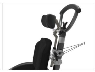
Figure 10: Adjusting the height of the head support
