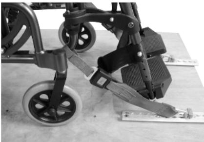
Fitting the front restraint
