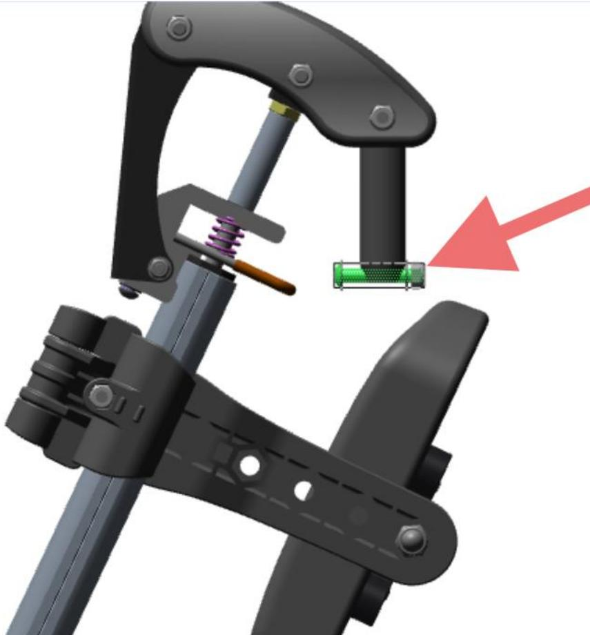
If the original screw set is missing, you may substitute it with standard M6 screws, washers, and nuts you have in stock.
