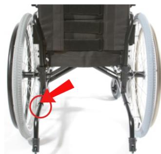
To fit: Depress rear location button on the antitip bar and slide into rear of frame tube. The front button **MUST** engage through the hole in the frame. Check antitip is secure by attempting to push backward and forward. Follow these instructions to fit the antitip bar on the other side of the wheelchair.
