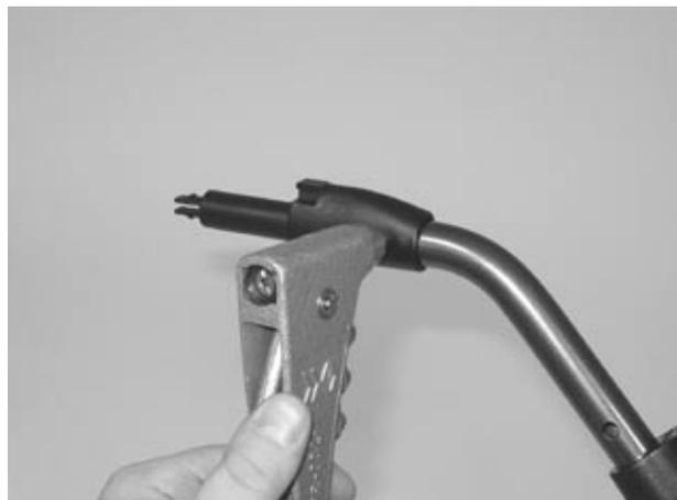
For re-assembly, plug all elements together and fasten the upper swivelling part using two rivets.
