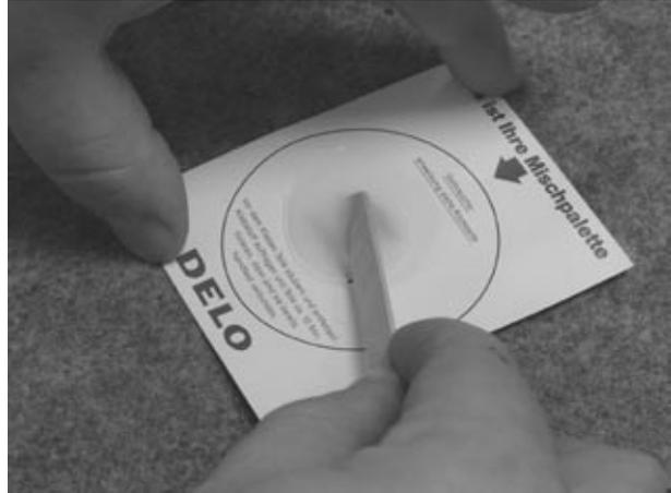
Open the two part adhesive sachet. Use the spatula to squeeze out all the contents of the sachet into the centre of the mixing card and mix the components for approx. 30 seconds.
