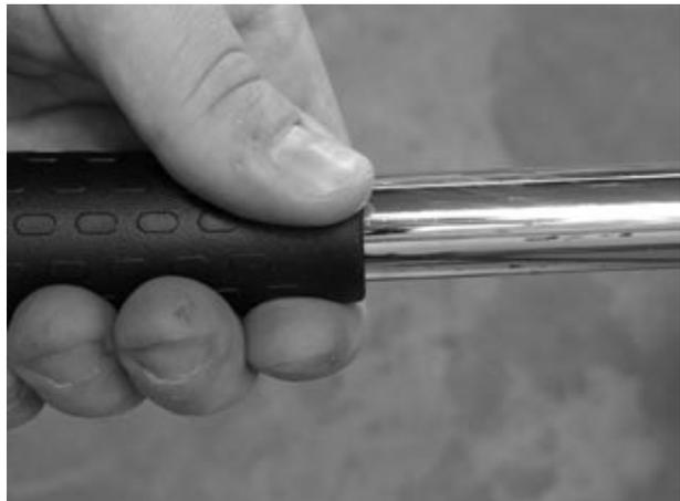
Slide the rubber hand grip onto the push handle rotating it through 180° as it is pushed on.
