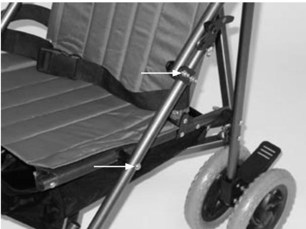
Next, loosen and remove the screw connections (Arrowed) between the anterior frame and the seat as well as between the anterior frame and the push handle.
