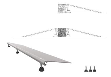
· Adjust the length of the adjustment feet to the desired wedge height
