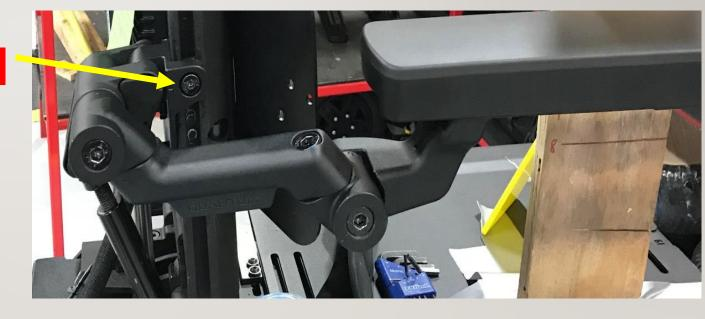
You will then need to loosen the 2 bolts under the Pillow block, loosen not take off
